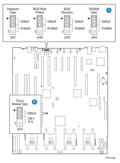
Figure 10. Mainboard Jumper Locations
